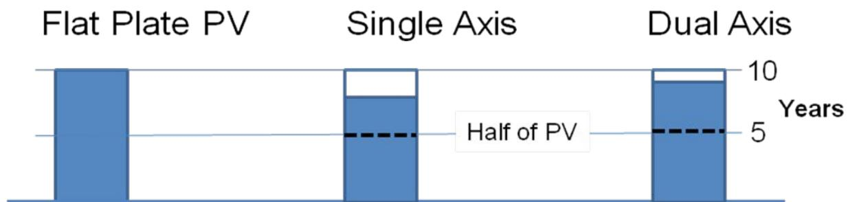
In a single axis hybrid, the savings are the same when heat and electricity are included. The annual savings are twice that of Flat Plate PV. But its BOM costs are also higher. Its payback is better than a dual axis hybrid though it does not meet the 5 year payback hybrid promise. Still, single axis hybrids are a sweet spot between flat plate PV and dual axis hybrids.
